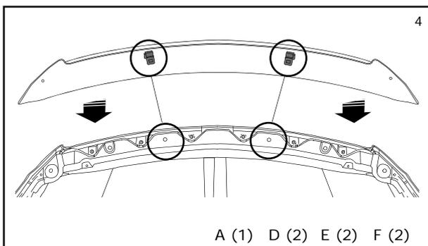
4. Re-fit hood protector to hood. Apply masking tape to hood underneath the square holes in the center metal clips. Mark the outline of the square hole onto the masking tape. Remove the hood protector.
